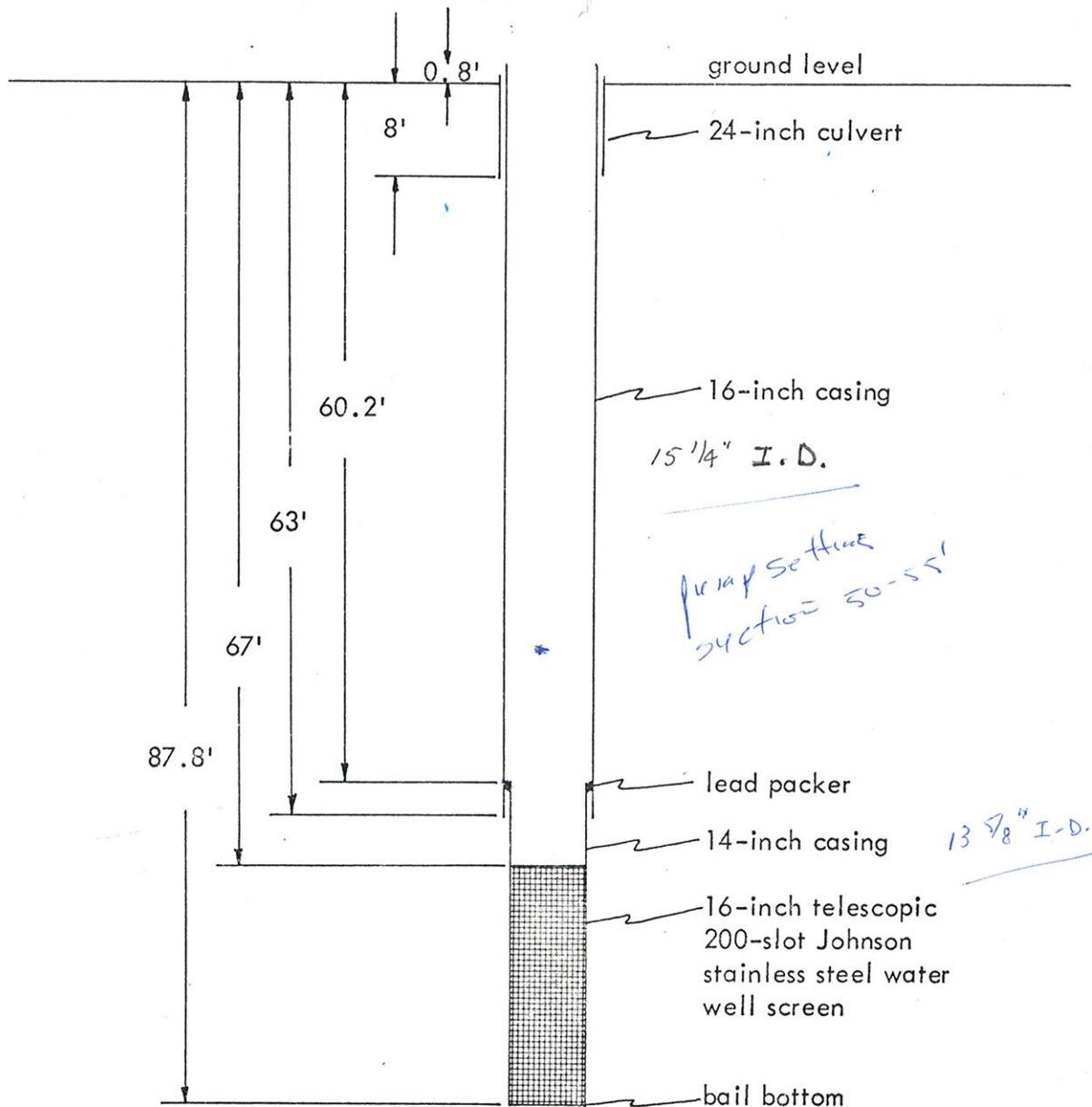
Figure 2. Completion diagram for Warm Water Well No. 6.
