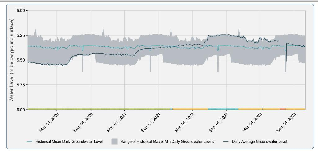
Max & Min data calculated from period of record from 2019–09–24 to 2023–11–01 (Date of last data entry) Smoothing applied to data: 7 day rolling mean
