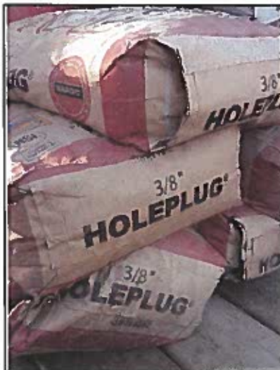
Photo 2. Bentonite chips used to seal GW4
