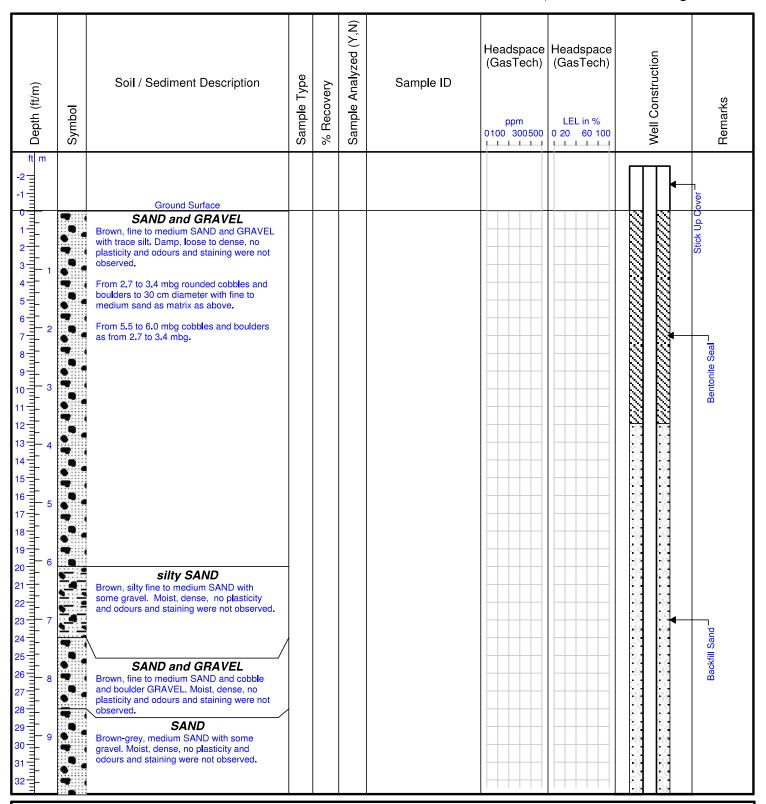
Date of Water Level: September 19, 2011 Water Level (from TOC): 17.27 m Well-Borehole Diameter: 22 cm Well Casing Diameter: 5 cm Well Casing Material: PVC
