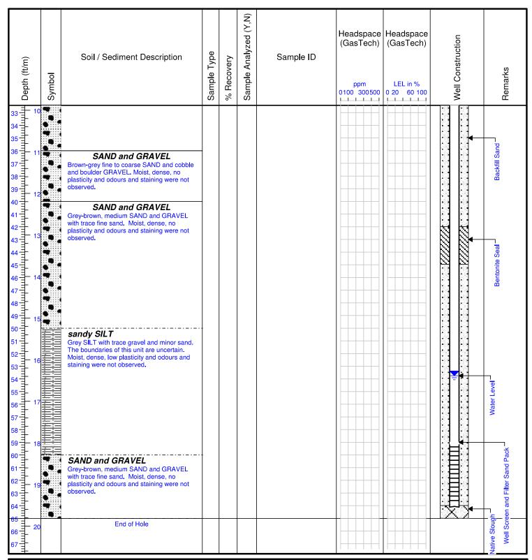
Date of Water Level: September 19, 2011 Water Level (from TOC): 17.27 m Well-Borehole Diameter: 22 cm Well Casing Diameter: 5 cm Well Casing Material: PVC Well Screen Slot Size: 10 Depth of Well (TOC): 20.5 m
