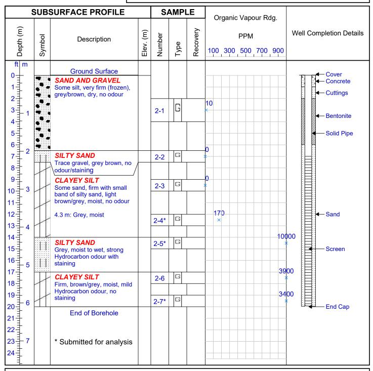
Drilled By: Hole Dia: 6" Well Dia: 2"
