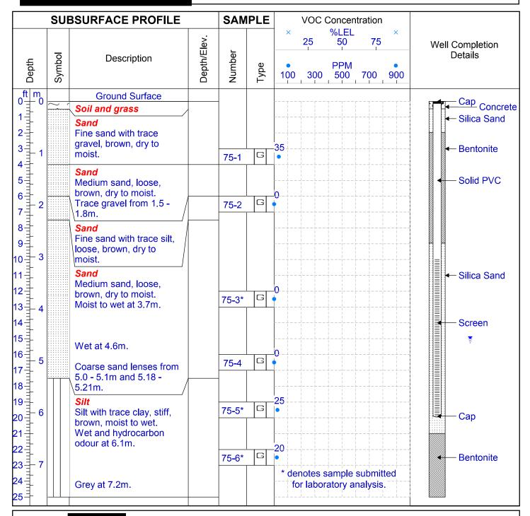
Drilled By Well Diameter: 2" Hole Diameter: 4"
