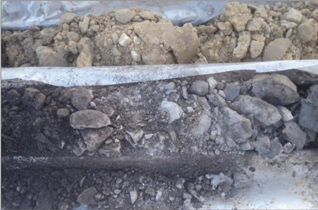
Photo 13: Organic rich shale encountered at 15MW06 at depth of 3.0 – 3.3 m bg. Photo taken on October 8, 2015 at 11:30 am.
