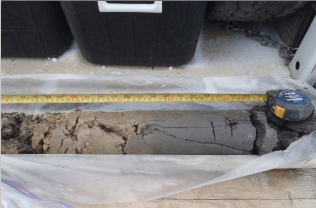
Photo 11: Saturated sand and gravel overlying fine grained silt and clay at 15MW04 at a depth of 0.7 to 1.5 m bg. Photo taken on October 7, 2015 at 2:30 pm.
