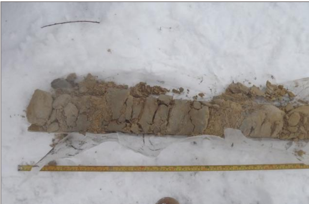
Photo 10: Sandstone encountered at 15MW03 (1.5 – 2.2 m bg). Photo taken on October 7, 2015 at 12:10 pm.
