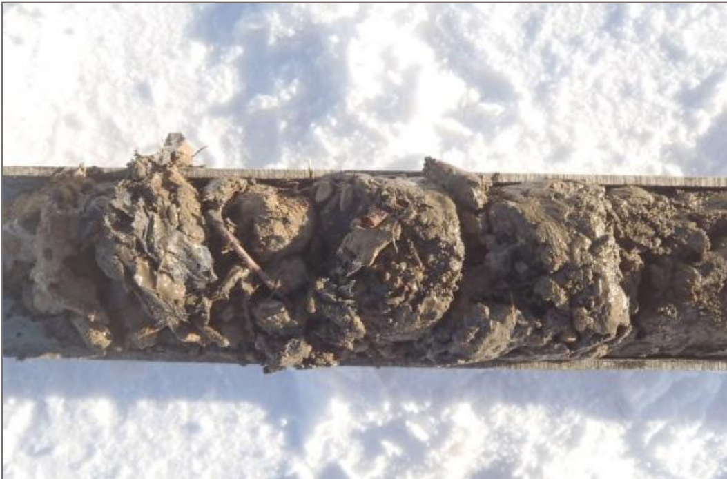
Photo 14: Organics, sand and gravel containing household garbage encountered at 15MW07 at a depth of 0 – 0.3 m bg. Photo taken on October 8, 2015 at 12:07 pm.
