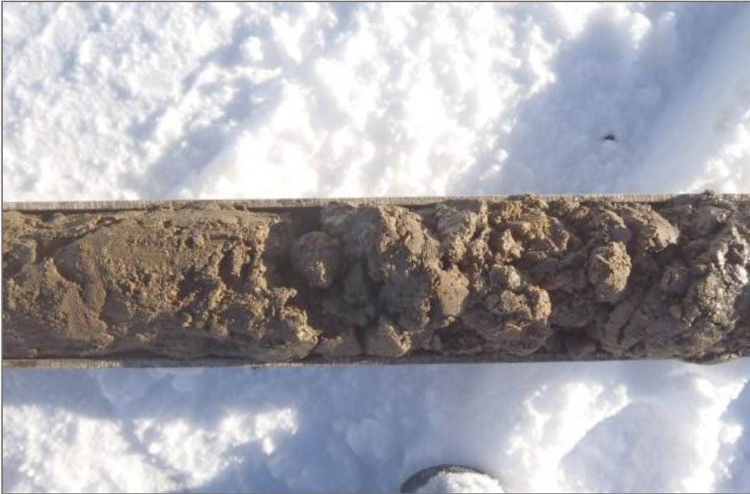
Photo 15: Moist to saturated sand and gravel overlying fine grained silt and clay encountered at 15MW07 at a depth of 0.6 – 1.2 m bg. Photo taken on October 8, 2015 at 12:07 pm.
