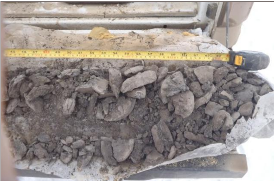
Photo 12: Organic rich shale bedrock encountered at 15MW01 a depth of 5.5 – 6.0 m bg. Photo taken October 7, 2015 at 4:12 pm.
