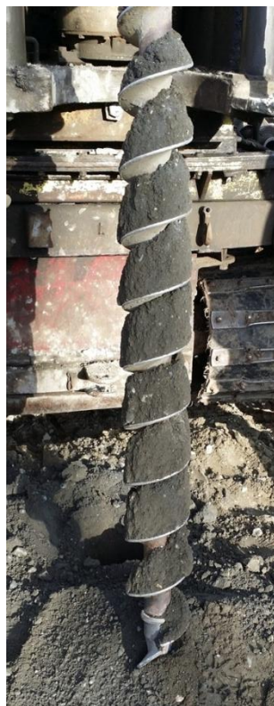
Above – Auger sample conditions. Till from 7.6 to 9.1 m
