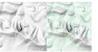
A canyon anomaly which has the potential of being an imposter watercourse. The anomaly turns out to be supported by the base data.
