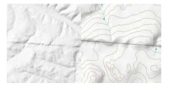
Edge effect due to lack of data If we desire a 'perfect' DEM our only option would be to make the area of interest smaller. The image on the left also shows a second source data error.
