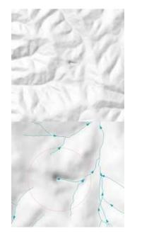
slope the elevations start to rise again. When compared with the adjacent tile to the south it is obvious the elevations should just continue smoothly downward.
